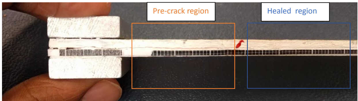
Figure 3-20 DCB sample of dual network epoxy with thiol healed at 90°C showing crack disappearance after the pre-crack region marked by red.
