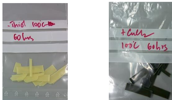
Figure 4-4 Free standing polymer samples showing difference in color after addition of CuCl 2
