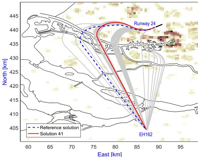
Fig. 6. Optimal ground tracks obtained in the first problem.
