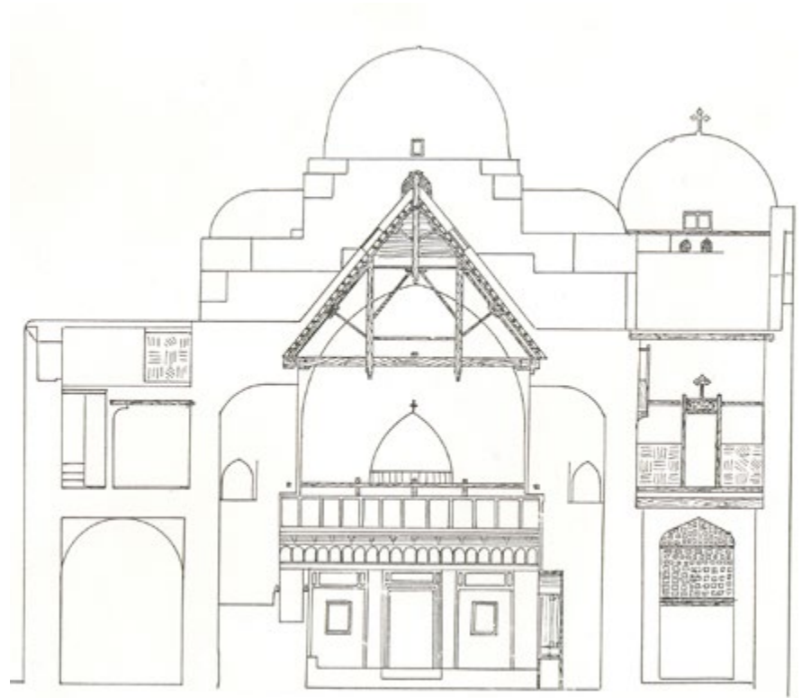
Figure 10: Cross section of St. Mercurius church highlighting the vault and the traditional skeleton of the Coptic church. Source: Maher Andraws, interview with author, January 14, 2025
