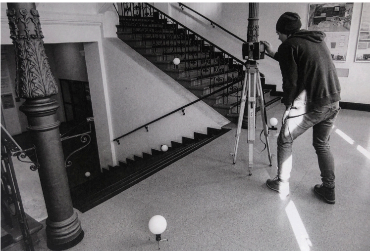
// 25 Static laser scanner with reference spheres.
