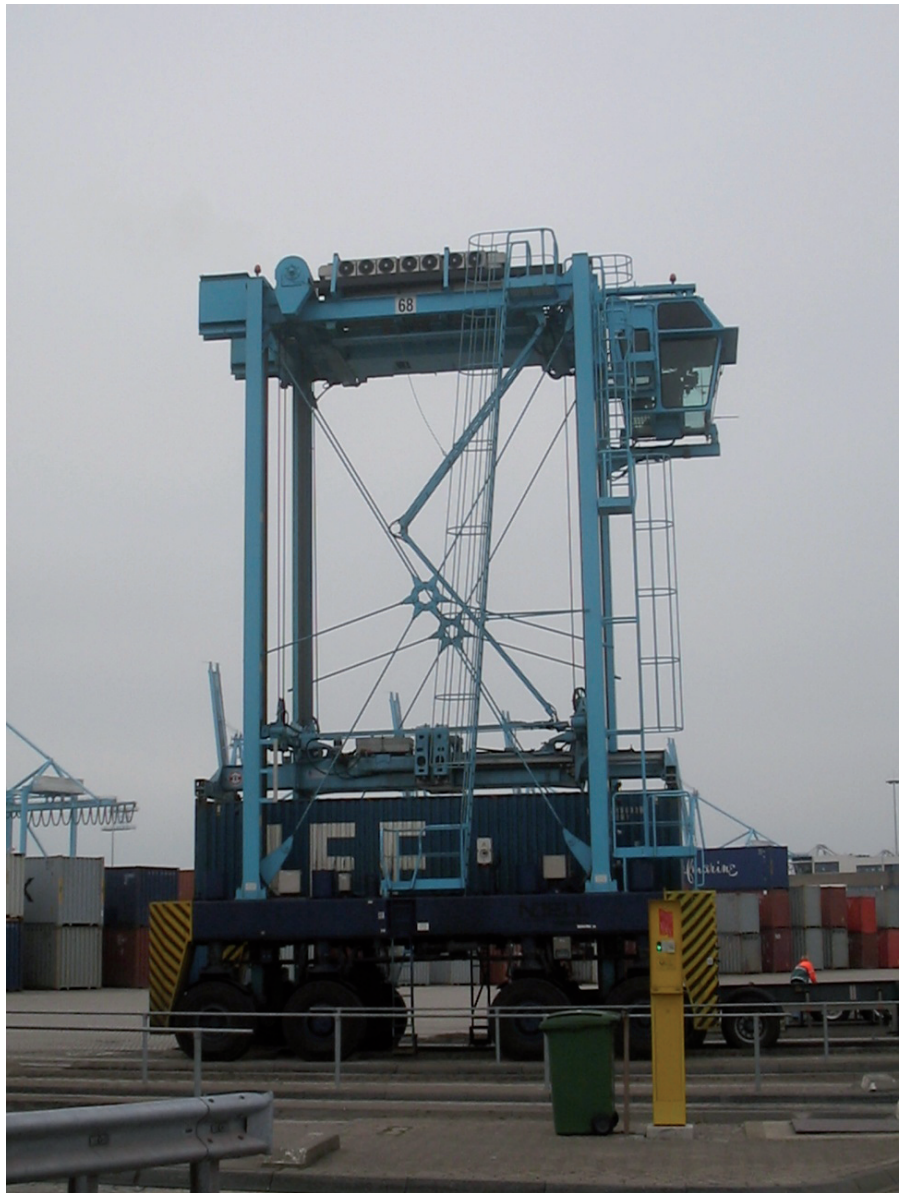
Figure 4.22: A straddle carrier [de Gijt ea 2003]
