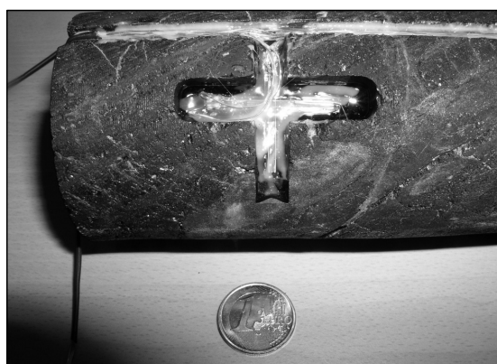
Fig. 5.1b Photo of strain gauges on the surface of the coal core
