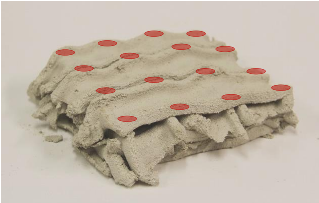
U-5 Nozzle , stacked, crossed extrusion
