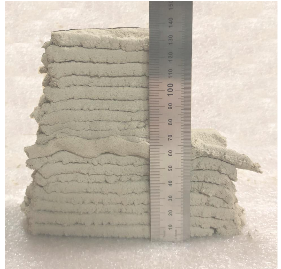
Dry mixture and wide flanges result in low compression
