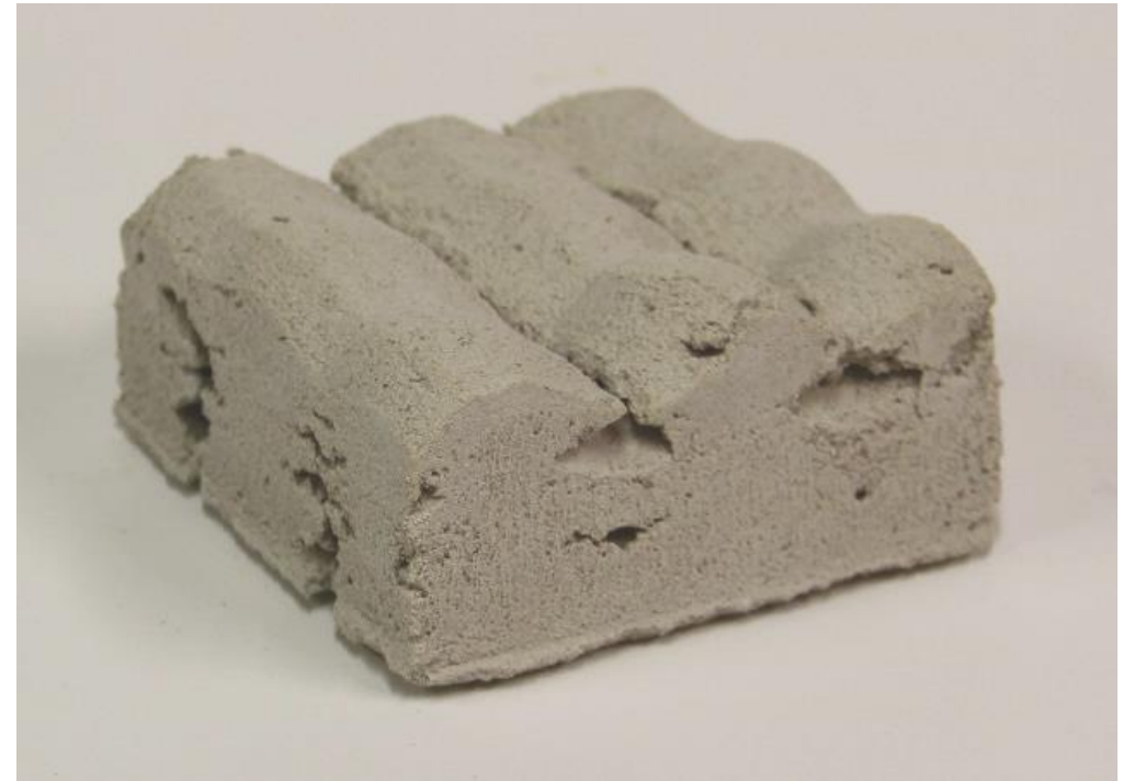
Triangular Nozzle, stacked, crossed-extrusion
