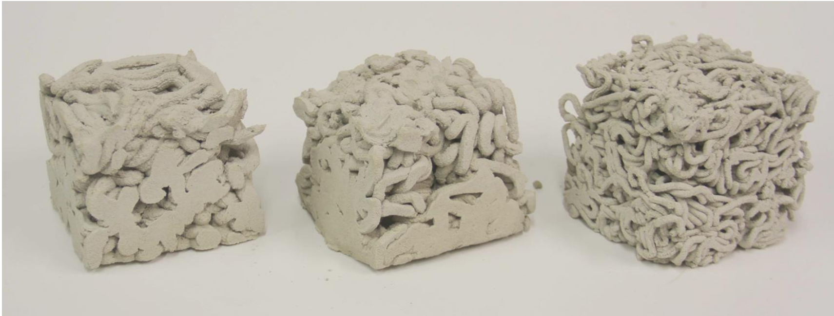
Compression due to self-weight is visible at the bottom
