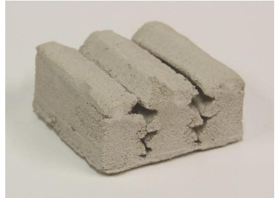
Load distribution over centre = stable extrusion
