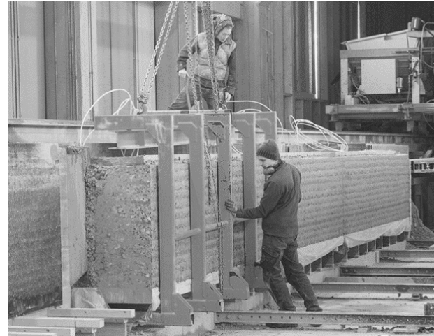
Eden, Rammed Earth Pre-Fab Element
