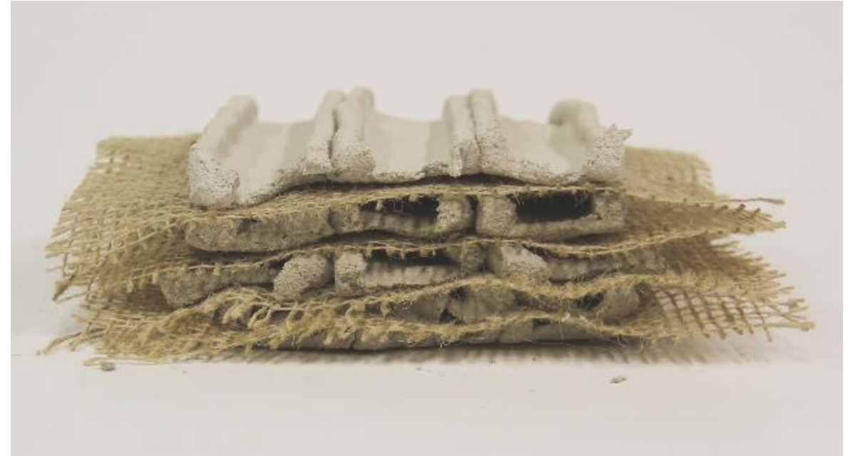
U-shaped straight extrusion with interlayer mesh
