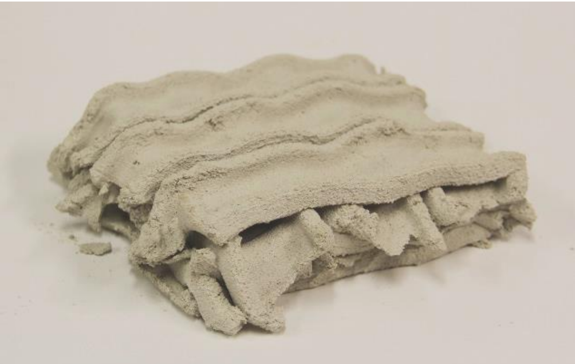
U-5 Nozzle , stacked, crossed-extrusion
