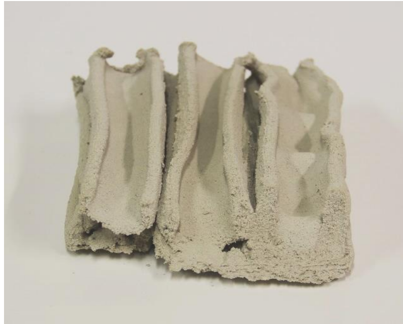
Narrow flange = unstable extrusion
