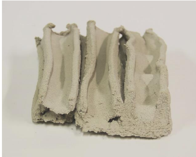
Narrow flange = unstable extrusion
