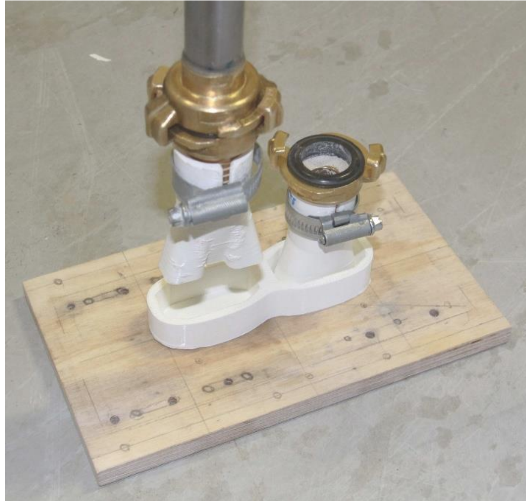
Automated nozzle change between several production steps
