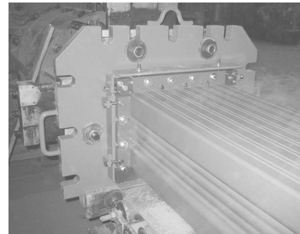
Conventional extrusion method for VPB
