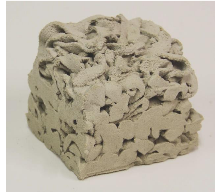
Enclosed air reduces the density
