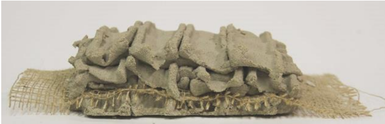
Compression due to self-weight and crossed toolpath induced point load
