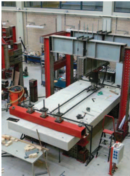
Figure 6. View of one of the Lantsoght slabs with a concentrated load nearby a support line
