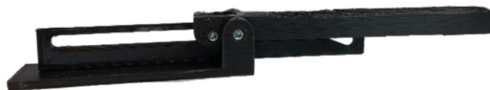
Figure 39: The prototype of the "blade slit" occlusion mechanism. In this configuration, the blade is positioned halfway.
