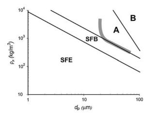
**Fig. 4** Modified Geldart's diagram (Valverde and Castellanos 2007b) showing the boundaries between the types of fluidization expected for fine particles, including solid-to-fluid like to elutriation (*SFE*) behavior and solid-to-fluid like to bubbling (*SFB*) behavior. The thick gray line represents the boundary between A and C powders as shown in the original Geldart's diagram (Geldart 1973)
