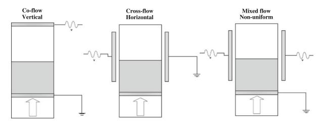
Fig. 8 Sketches of the three different setups used in the alternating electric field enhanced fluidization:  $\mathbf{a}$  co-flow electric field,  $\mathbf{b}$  cross-flow electric field,  $\mathbf{c}$  variable electric field (reprinted from Lepek et al. (2010) with permission from Wiley)
