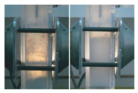
**Fig. 9** Snapshots of a fluidized bed of unsieved R974 silica before (*left*) and after (*right*) the electric field was applied (variable field configuration) (reprinted from Lepek et al. (2010) with permission from Wiley)
