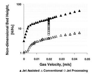
**Fig. 10** Comparison of the non-dimensional fluidized bed height as a function of gas velocity for conventional and microjet-assisted fluidization of Aerosil R974 (reprinted from Quevedo et al. (2010) with permission from Wiley)
