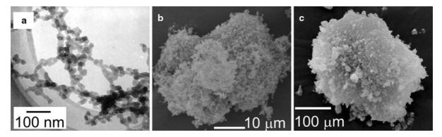
Fig. 3 Illustration of the multistage agglomerate structure obtained by ex-situ analysis. a TEM image of a network of silica NPs. b SEM image of a simple agglomerate or sub-agglomerate built up from these networks. c SEM image of a
