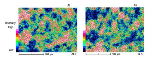
Fig. 12 Element mapping images of film surface of mixing sample ( $G_0 = 40$ ;  $U_0/\text{Umf} = 1.5$ ; SEM magnification was 1,000 times; mixing time was 6 min) (reprinted from Nakamura and Watano (2008) with permission from Elsevier)
