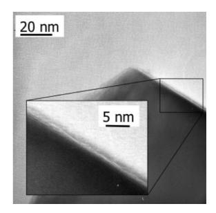
Fig. 13 TEM picture of a  $LiMn_2O_4$  particle coated with a thin layer of alumina (five ALD cycles) at atmospheric pressure. Such NPs can be used as cathode material in Li-ion batteries (reprinted from van Ommen et al. (2010b) with permission from Elsevier)
