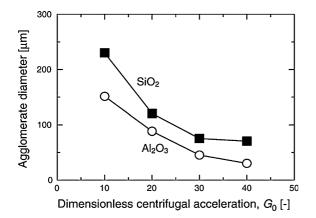
**Fig. 6** Agglomerate size of nano-particles as a function of centrifugal acceleration for a Richardson and Zaki exponent n = 5 (reprinted from Nakamura and Watano (2008) with permission from Elsevier)
