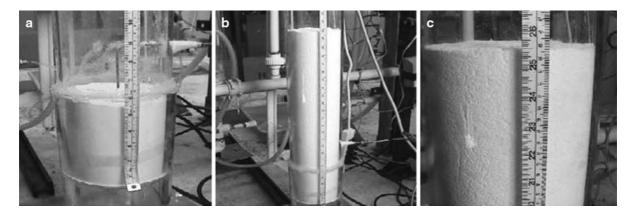
**Fig. 11** Images corresponding to the fluidization of Aeroxide  $TiO_2$  P25 in a 5-inch (12.7 cm) ID column. **a** Initial bed height, **b** maximum bed height when fluidized with microjet assistance, and **c** close-up of the fluidized bed surface. The fluidized bed
