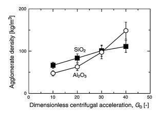
**Fig. 7** NP agglomerate density as a function of centrifugal acceleration. *Error bars* the differences with a change of n in a range of 4–6 (reprinted from Nakamura and Watano (2008) with permission from Elsevier)
