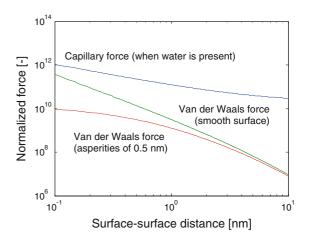
**Fig. 1** The main forces between two silica particles of 10 nm as a function of the interparticle distance. All forces are normalized by dividing them by the gravity forces on a single particle. The capillary force is given for water; for other liquids, this force is typically lower. The van der Waals force depends on the surface roughness, as shown by the curves for a smooth surface and for surface asperities. Models and constants from Butt and Kappl (2010)
