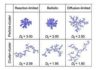
Fig. 2 Kinetic growth models in a 2D embedding space. The mass fractal dimension D of their 3D analogs are given (based on Friedlander (2000))
