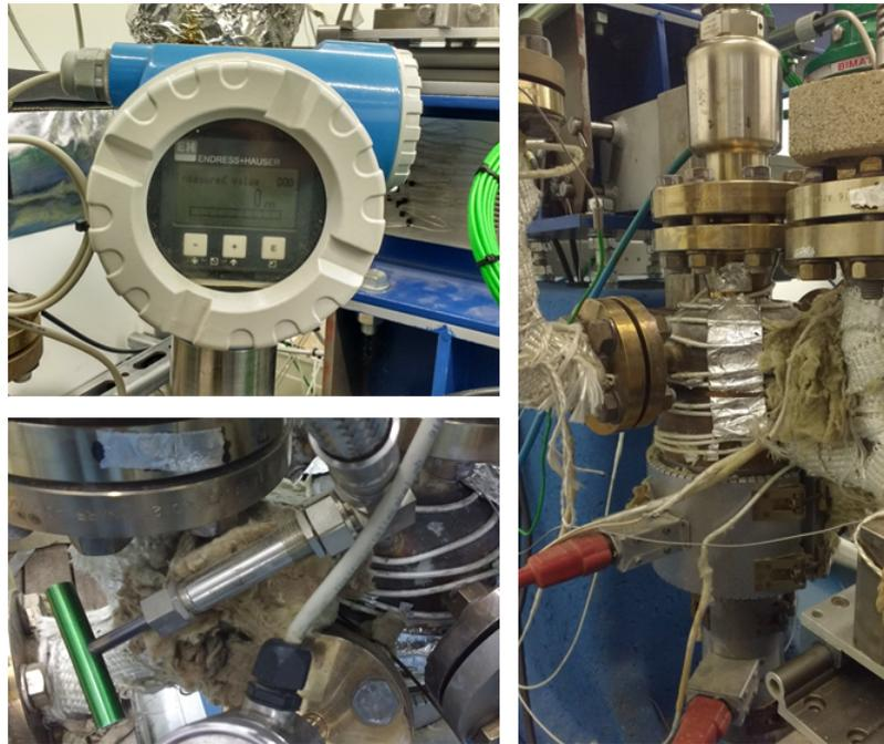
Figure A.5: Image of the vapour generator HFT-1 (right) with the liquid level indicator LIT1 (top left) and valve MV2 (bottom left)
