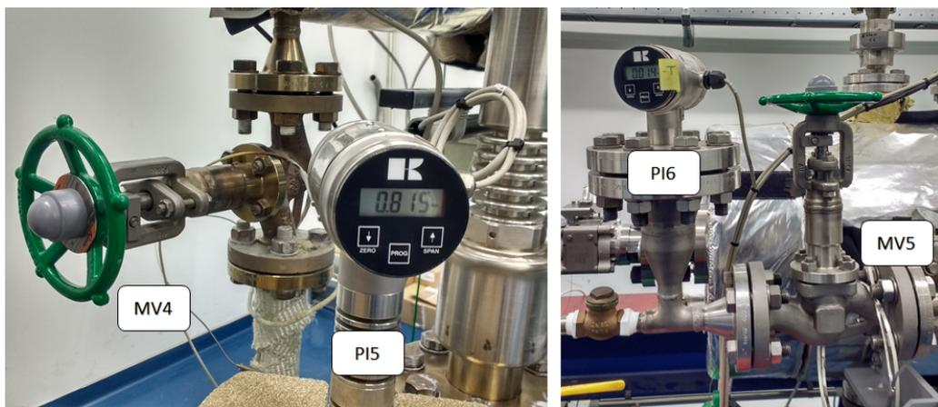
Figure A.3: Image of the manual valves and pressure sensors MV4, PI5 (left) and MV5, PI6 (right)
