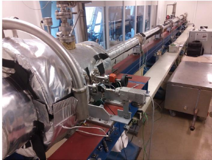
Figure 3.2: Flexible Asymmetric Shock Tube setup commissioned at TU Delft [8]
