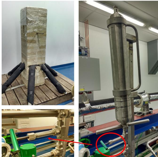
Figure A.4: Image showing the siloxane container (top left), the swagelok FFC-1 botte (right) and valve MV1 (bottom left)
