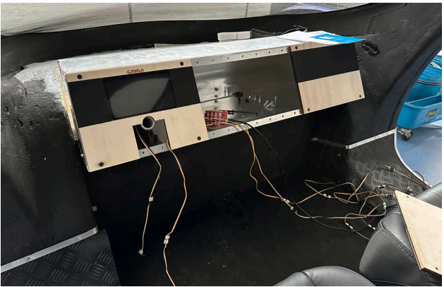
Figure 55: Wiring behind the dashboard to make the steering wheel prototype work.
