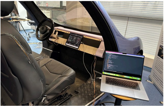
Figure 56: Steering wheel prototype embedded in the car with the Arduino code.
