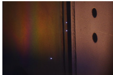
Figure 5.90: Discharge sparks on the vacuum chamber inside walls
