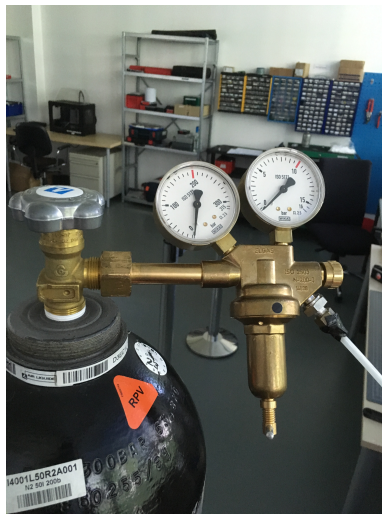
Figure 6.3: Pressure reliever and nitrogen flow regulator
