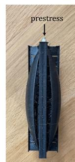
Fig. 12: Using a threaded rod and nuts to prestress VTS element.
