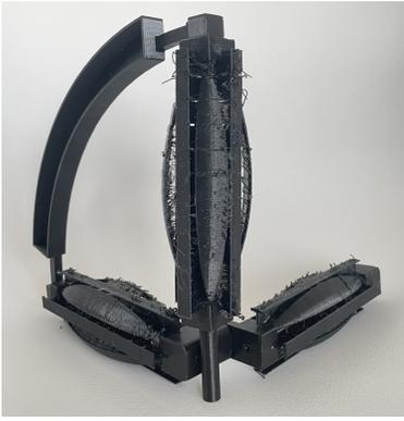
Fig. 29: Fabricated compliant VS ball joint.
