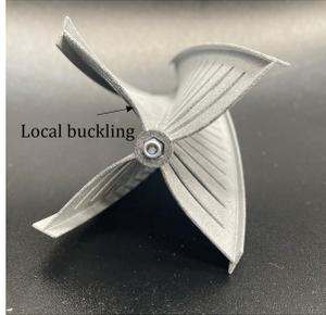
Fig. 19: Local buckling of the T beam.
