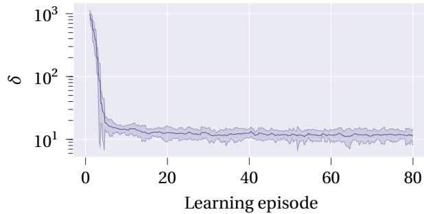
Figure 6.6.: Moving average of the TD error during the learning process (window length = 239, i.e., number of transitions per episode)
