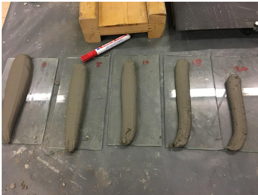
Fig. 5. 29: S20 paste mixture with 0.75% Acti-gel and l/b-ratio of 0.315
