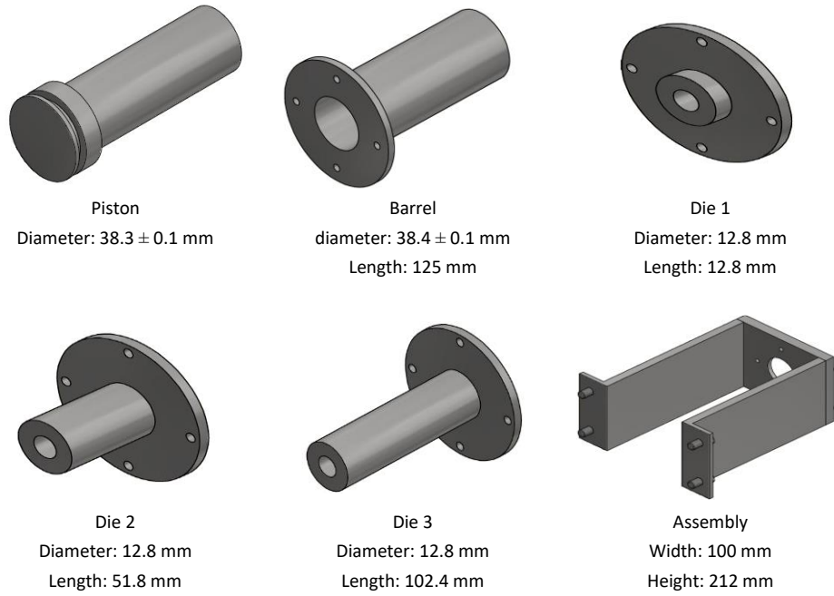
Fig. 5. 11: Ram extruder components
