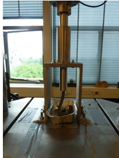
Fig. 5. 13: Example of Ram extruder paste extrusion
