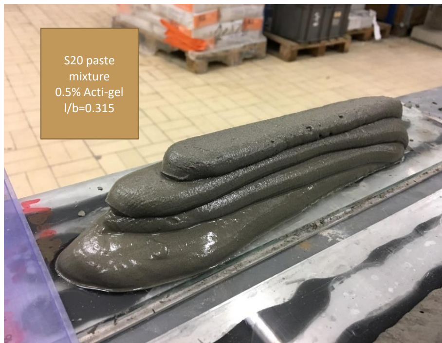
Fig. 5. 26: 4 layers of S20 paste mixture with 0.5% Acti-gel
