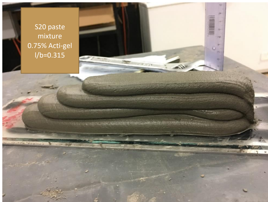
Fig. 5. 27: 4 layers of S20 paste mixture with 0.75% Acti-gel
