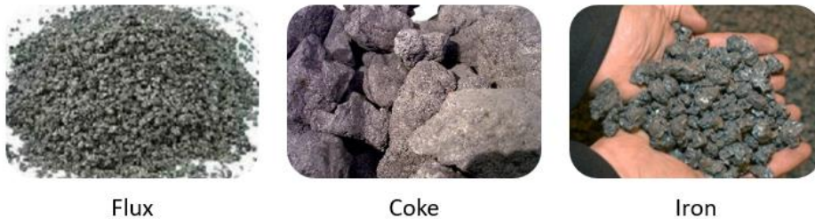
Fig. 3. 4: Raw components for the formation of BFS [47] [48] [49]
