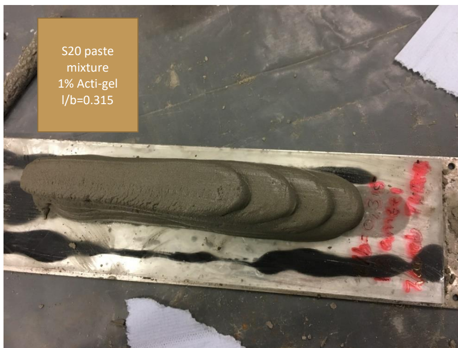
Fig. 5. 28: 4 layers of S20 paste mixture with 1% Acti-gel
