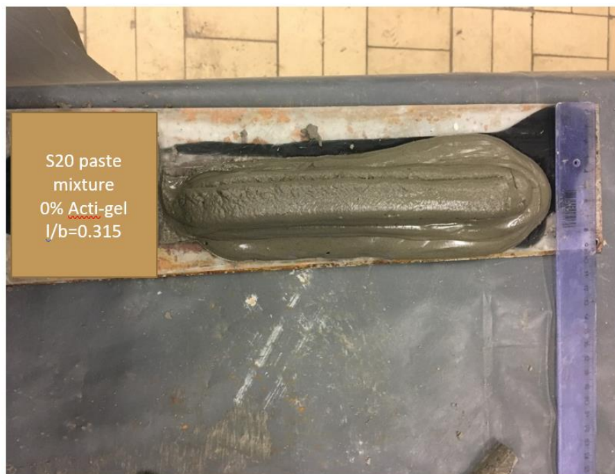
Fig. 5. 25: 4 layers of S20 paste mixture with 0% Acti-gel
