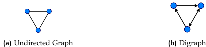
Figure 1.3: A undirected graph and a directed graph with both 3 vertices and edges as connections between the vertices [Wikimedia Commons, 2007a] [Wikimedia Commons, 2007b]
