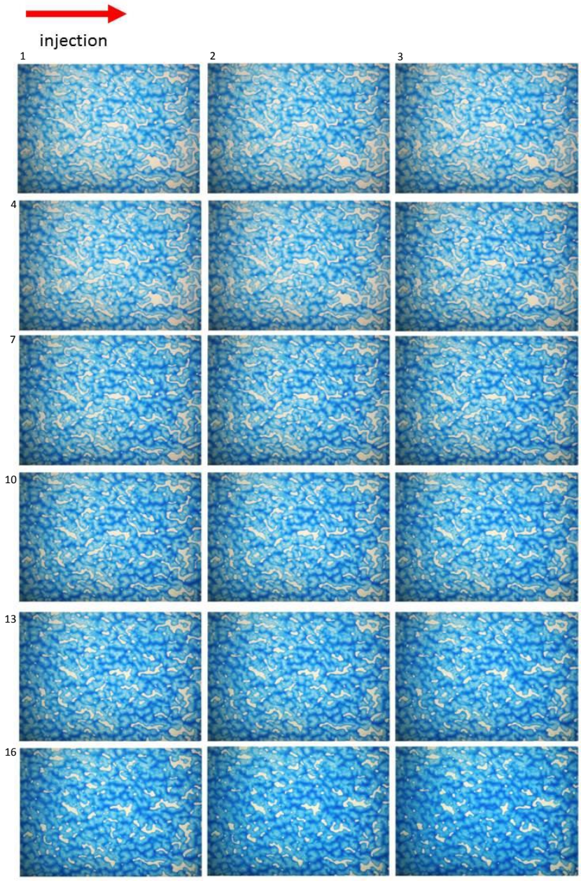
Figure 2.9: Capillary-desaturation experiment of Sample 4 (unprocessed Images)
