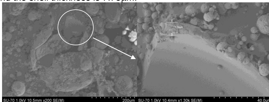
Figure 3: SEM images of a broken microcapsule showing its inner structure.
