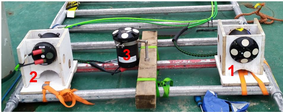
Figure 3.26: Photo of ADCP1 (right), ADCP2 (left) and ADCP3 (middle). ADCP1 and ADCP2 are horizontally mounted within a wooden structure attached to the measurement frame. ADCP3 is mounted looking vertically upwards by means of a clam to the measurement frame.
