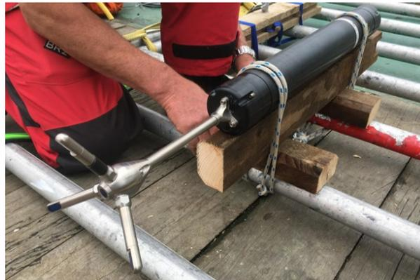
Figure 3.24: Photo of ADV4 mounted on the horizontal measurement frame. Apposed to ADV 1-3, ADV4 has a fixed stem between the head and the case. Thus, the head could not be placed in the same manner as ADV 1-3 illustrated in Figure 3.23. The head of ADV4 is rotated 90° in anti-clockwise direction compared to ADV 1-3 with the positive x-axis (black band around ADV arm) directed upwards in positive z-direction according to the reference system.
