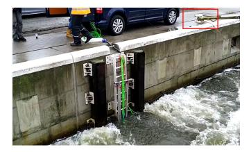
Figure 3.18: The white stairs located 4 m away from bollard 28 (red box) which were used as reference point for the measurement. The top scaffolding of the vertical frame is mounted on the stairs for support. The green cables in the figure are the instrument cables from the pressure sensors, ADVs and ADCPs.
