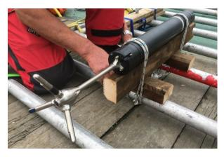
Figure 3.24: Photo of ADV4 mounted on the horizontal measurement frame. Apposed to ADV 1-3, ADV4 has a fixed stem between the head and the case. Thus, the head could not be placed in the same manner as ADV 1-3 illustrated in Figure 3.23. The head of ADV4 is rotated 90° in anti-clockwise direction compared to ADV 1-3 with the positive x-axis (black band around ADV arm) directed upwards in positive z-direction according to the reference system.
