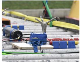
(a) Illustration of the flexible head ADV (1-3) while mounted on the horizontal measurement frame. In white the wooden structure holding the ADV in place is illustrated. In red the sampling volume of the ADV is illustrated. The total height above the bed at which the ADV measures the flow velocities is 0.357 m.
