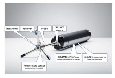
Figure 3.8: Illustration of the Nortek Vector ADV. The probe (head of the ADV) consists out of the transmitter in the centre, which sends out the sound pulses, three receiver arms, that listen to the echo of the sound pulses, and the temperature sensor. The case (housing of the ADV in black) consists out of the pressure sensor, tilt sensor, magnetometer and compass (Nortek Manuals, 2018a).
