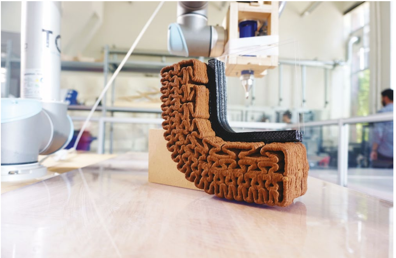
Figure 10: Final 3D-printed window frame.
