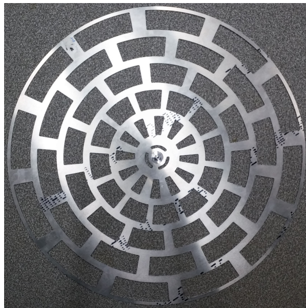
Figure 9.3: Mesh Design 1c: Porous Disc with large punctured holes.
