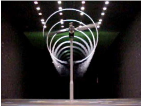
(a) Wake of a two-bladed 10 m diameter horizontal axis wind turbine [56]
