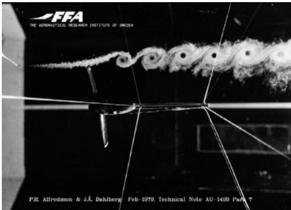
Figure 3.4: Flow Visualisation of the Tip Vortices of a 2 Bladed Rotor [3] .
