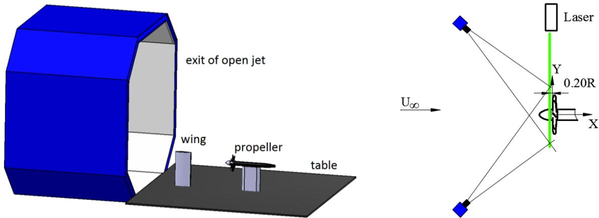
**Figure 6.** The experimental setup of the propeller blade vortex interaction (left) and a top view of the PIV setup in the upstream plane perpendicular to the propeller axis (right). Figure reproduced from Yang (2017).
