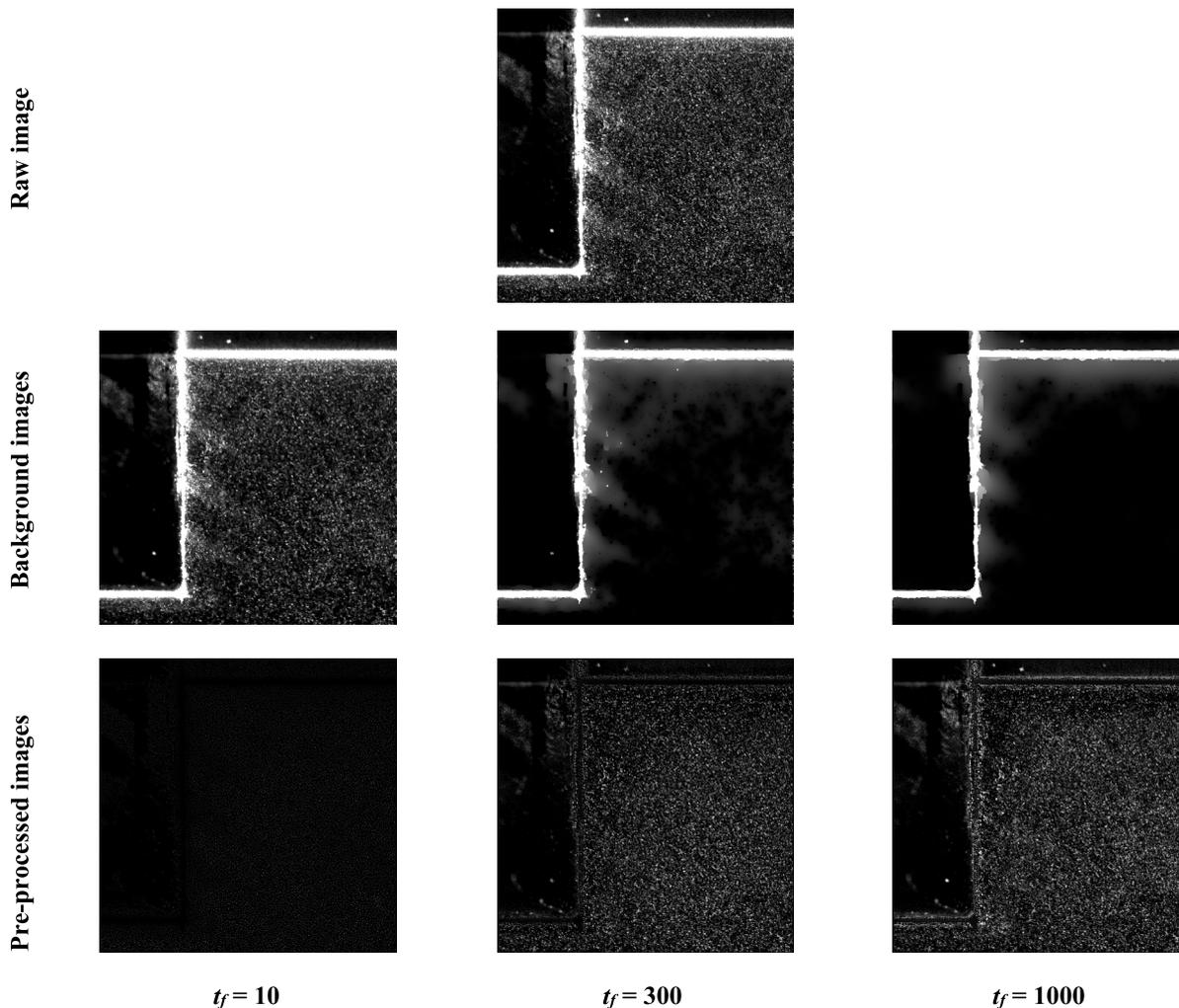
**Figure 4.** A comparison of background and pre-processed images obtained using the proposed anisotropic diffusion approach with  $K = 10$  after different numbers of iterations ( $t_f = 10, 300, 1000$ ).
