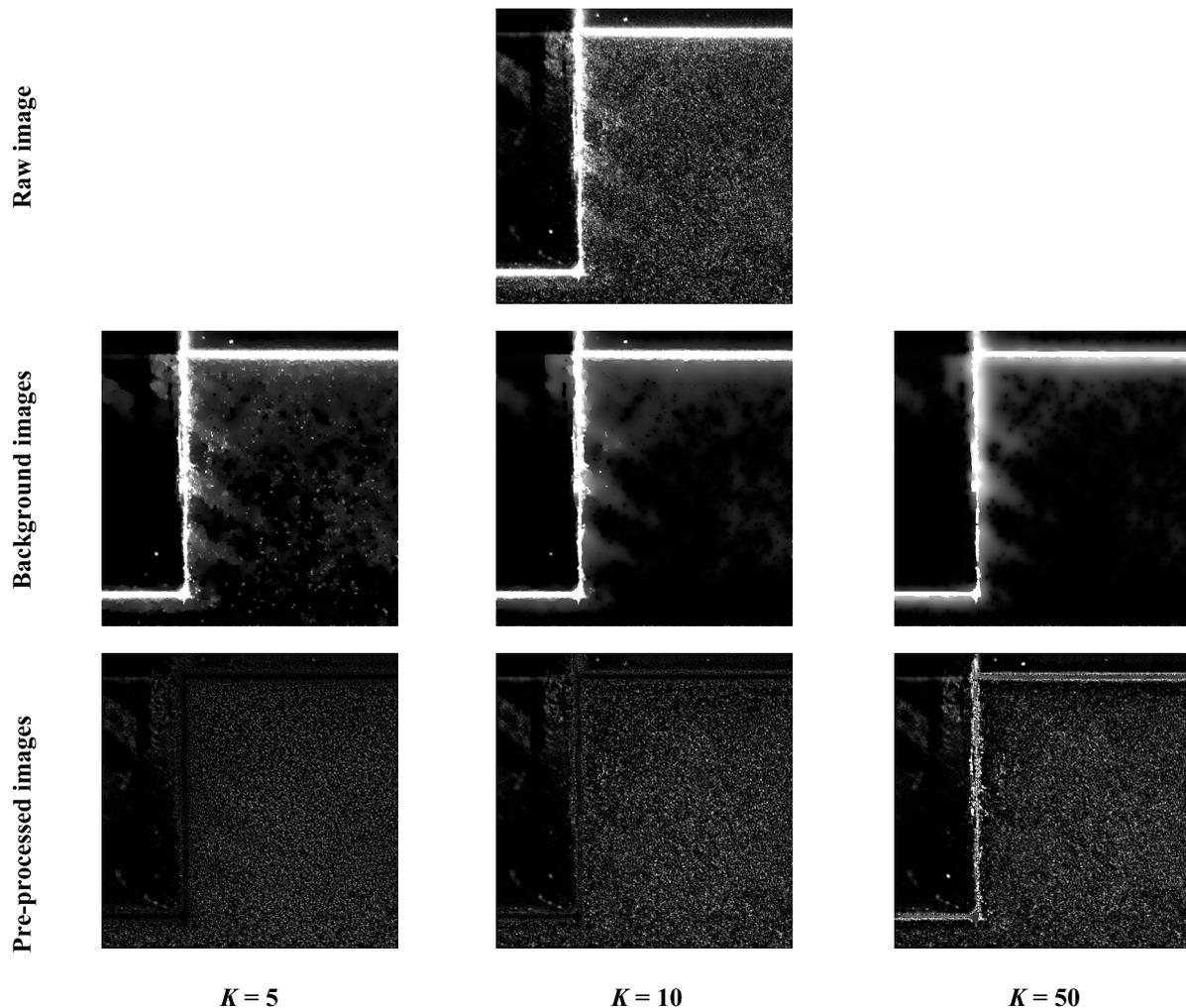
**Figure 3.** A comparison of a raw image (top row), background images obtained using the proposed anisotropic diffusion approach after 300 iterations (middle row) and the pre-processed images for different values of the threshold parameter ( $K = 5, 10, 50$ ; bottom row).
