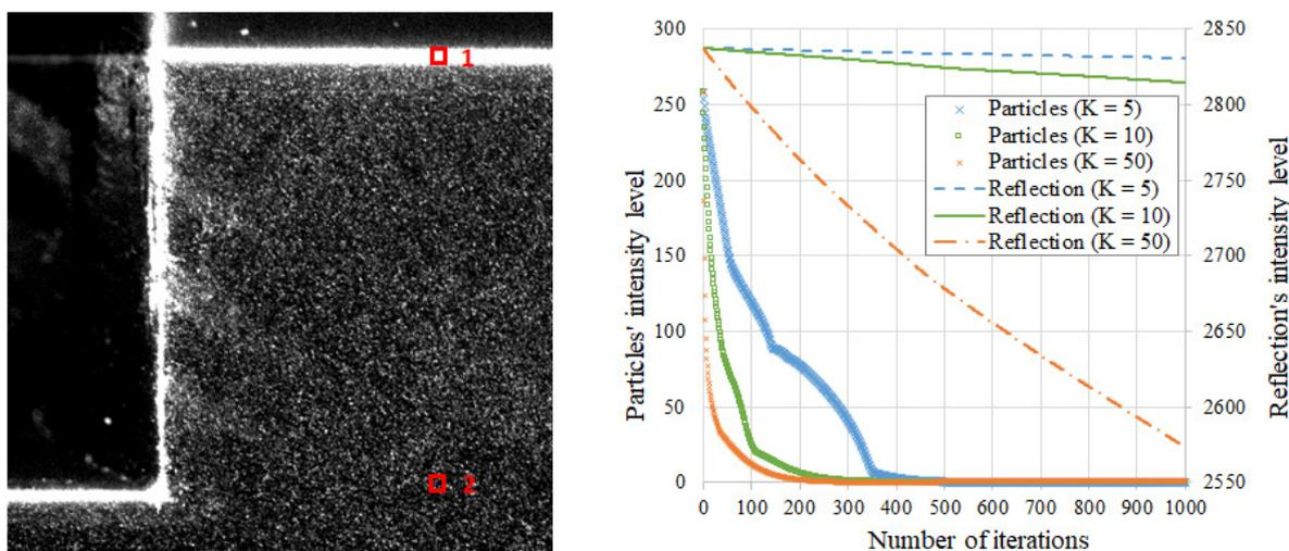
**Figure 5.** A plot of the intensity levels of particle images and reflection in the background image versus the number of iterations in the proposed anisotropic diffusion approach with different values of  $K$  (the areas where the reflections' and particle images' intensities are analyzed are the red squares 1 and 2 in the figure on the left, respectively).
