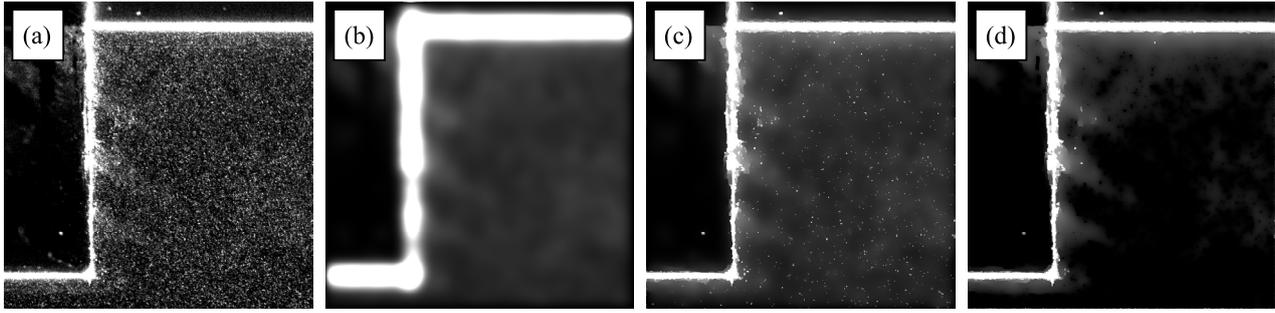
**Figure 1.** A comparison of different approaches for retrieving the background image. (a) A raw image of a cavity flow measurement (Iannetta *et al* 2016); (b) a background image by isotropic diffusion (sliding-average intensity); (c) a background image by the Perona and Malik (1990) approach; (d) a background image by the proposed approach. The following parameter values are used for the evaluation of the background image:  $K = 10$  and  $t_f = 300$ ,  $t_f$  being the number of iterations.
