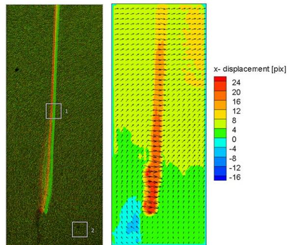
**Figure 7.** A raw image pair (left; red: first recording and green: second recording) and the corresponding displacement field (right). The interrogation windows where the cross-correlation analysis is conducted are shown in the raw image pair.
