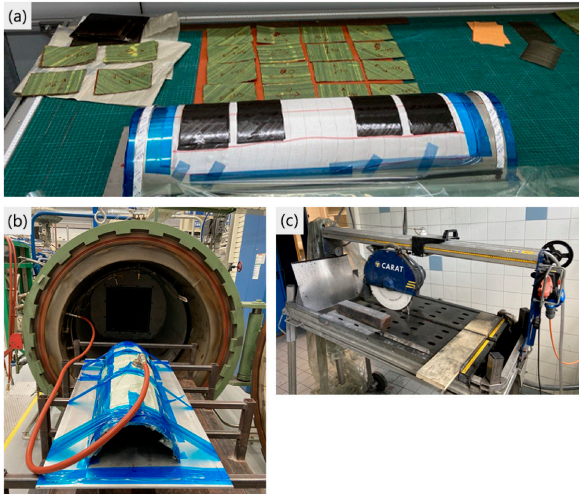
Figure 1. Different manufacturing stages of the curved composite panels: (a) a flat metal sheet transformed into a curved mould with desired curvature radius (13 cm) to stack the layers that were cut into standard dimensions, (b) the autoclave was set up according to the curing cycle of the preregs, (c) the edges of the cured samples were trimmed using a cutting machine to achieve precise dimensions and smooth edge finish.
