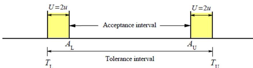
Figure 2.9: Two-sided acceptance interval with guard bands indicated in yellow. The tolerance interval is the interval in which the quantity is desired to be. The guard band is a buffer zone to account for uncertainty in measured values. Only values in the acceptance interval are accepted. Figure taken from the GUM (2012).
