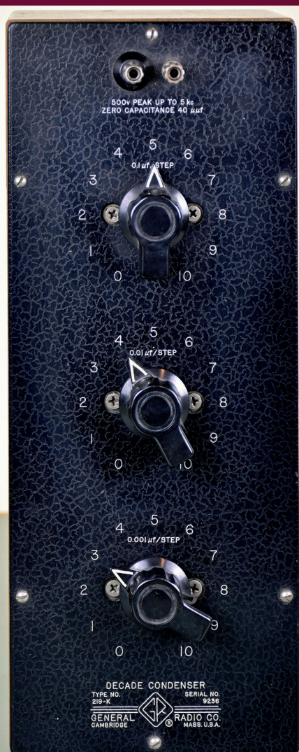
Figure 7. Decade condenser (Capacitor)
