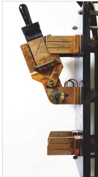
Figure 1. at the closing switch, the tension of the springs causes a quick separation of the contacts
