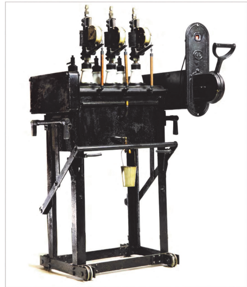
Figure 2. The use of oil as isolation medium for a more compact construction of power switches. (Photo: QOC Utrecht)
