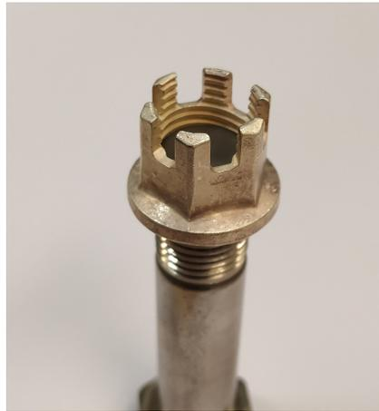
Figure 2.11: Castellated nut partially screwed onto a bolt.
