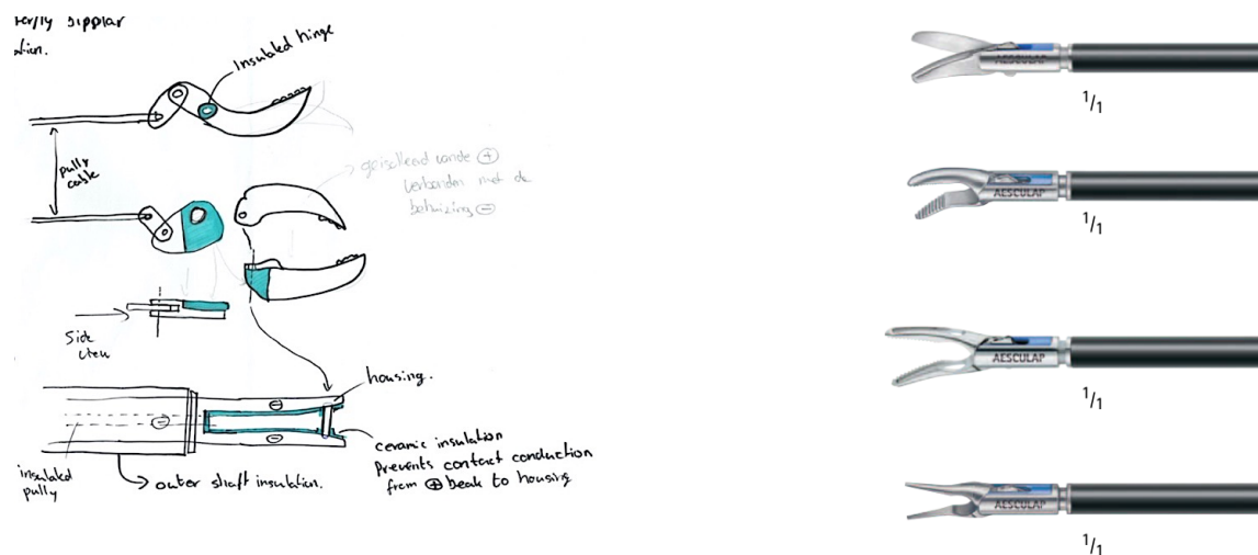
Figure 2-5, AdTec instrument(s). Left: sketch of an exploded view of the instrument. The ceramic insulation layers are coloured in cyan. Right: various reusable AdTec instruments with different functionalities [33]. The ceramic material is coloured blue. Note that these are bipolar laparoscopic instruments, but not specifically vessel sealers.
