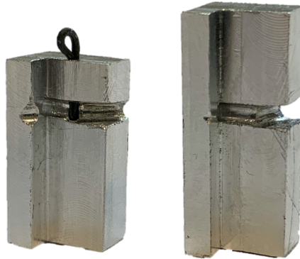
Figure 6-4, Aluminium 'angle blocks'. Left: 45 degrees angle at slider High side with hinge axis pin. Right: 70 degrees angle at slider low and H hinge side. There is no interference of the hinge pin while steering in this direction.
