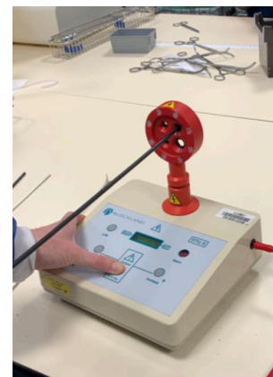
Figure 2-3, Insulation testing. Using a PTU6 pinhole detector the CSSD staff can easily check the electrical insulating components for insulation failure.
