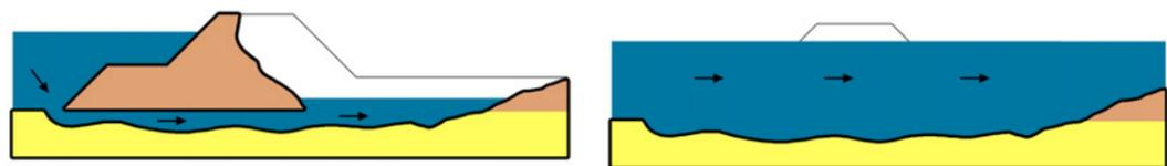
(a) Phase 4: Cracking and deformation of dike (Vandenboer et al., 2018). (b) Phase 4: Dike breach (dike failure) (Vandenboer et al., 2018).
