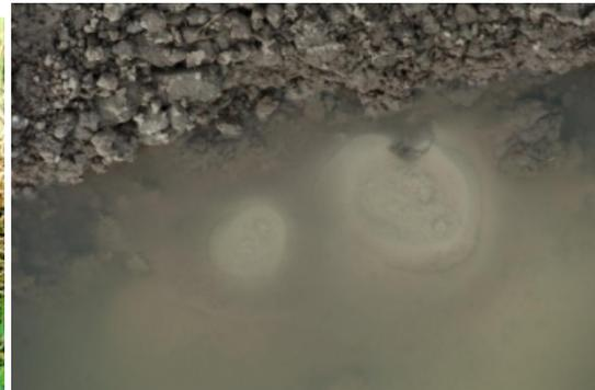
(b) Due to a further increase in hydraulic head, the sand fluidizes and becomes mobile, sand is deposited and forms shape similar to a well (de Bruijn, 2013).
