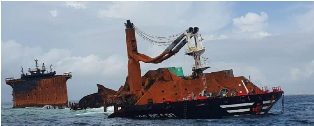
Figure 1.5: X-press pearl after the engine room flooded as a result of a fire [22]
