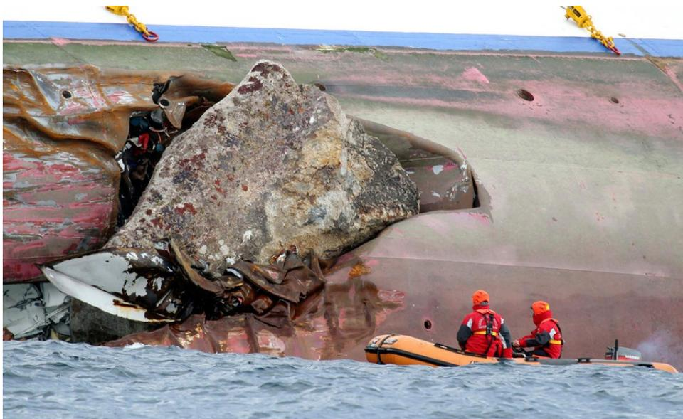
Figure 1.4: Wreck of the cruise ship Costa Concordia with the rock that caused the ship to flood [18]
