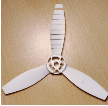
Fig. 37 Damaged propeller with BD=10\% .
