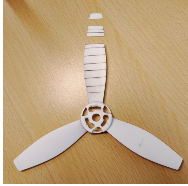
Fig. 38 Damaged propeller with BD=25\% .
