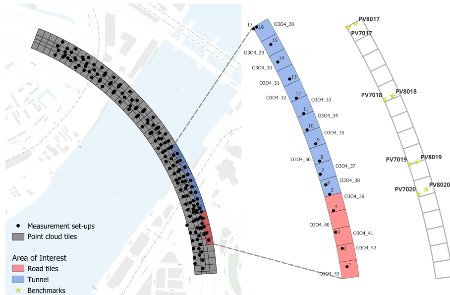
Figure 3.4. TLS measurement set-ups, sub-division tiles, AoI and benchmarks
