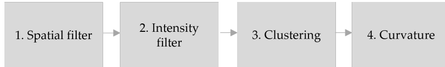
Figure 4.21. Schematic overview steps extraction points spherical targets
