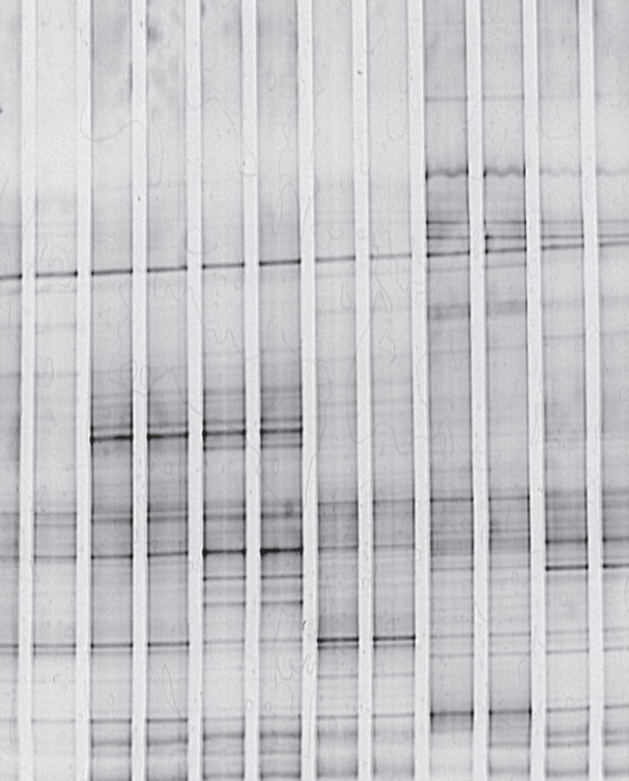
DGGE banding profile of the samples from SBRs subjected to increasing salinity
