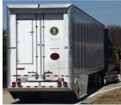
**Figure 2.7:** circulation control applied to a truck by Englar [45]
