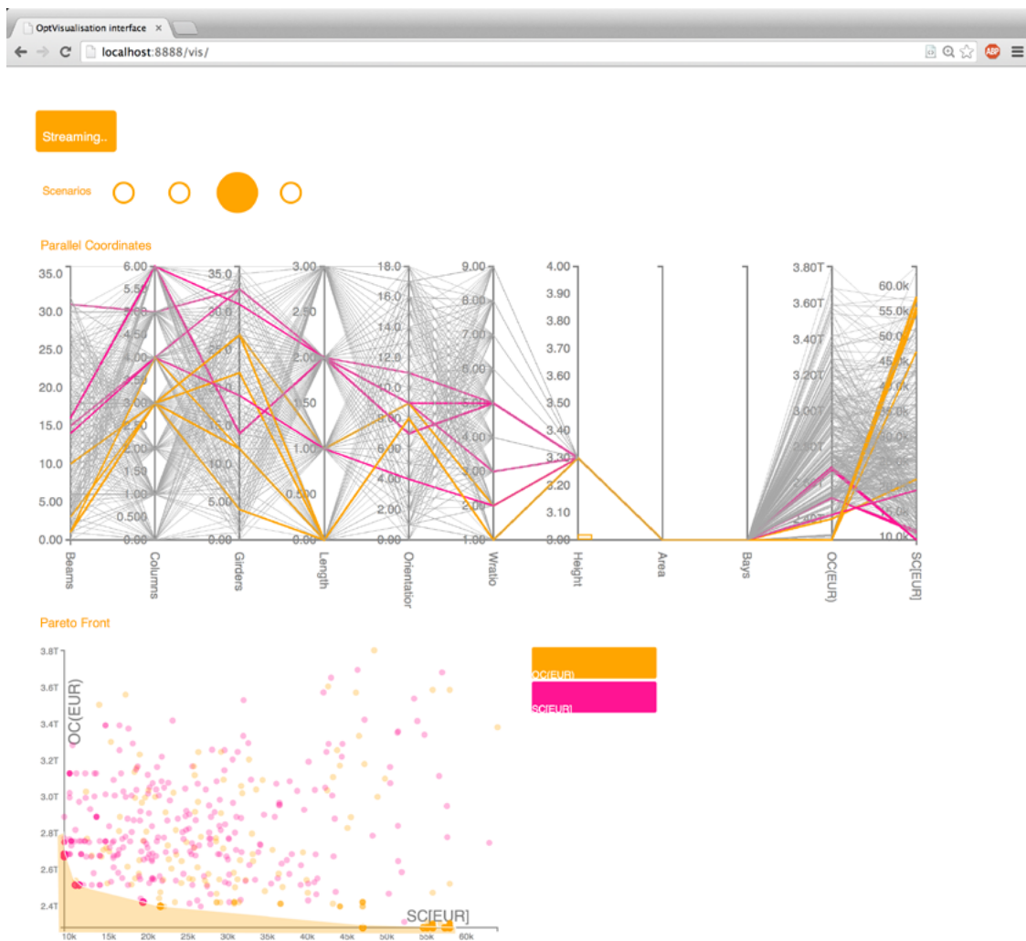
Figure 6. Interactive optimisation interface for investigating scenarios using parallel coordinates and objective graphs to investigate Pareto optimal fronts. Dataset: result of multidisciplinary optimisation benchmark of structural (SC) and operational costs (EC) of a classroom building.
