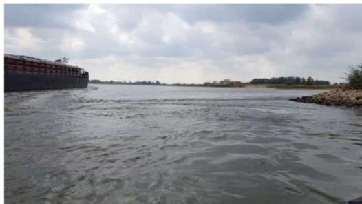
Figure 3. Video still of flow caused by ship sailing from the IJssel downstream of the bifurcation into the Nederrijn upstream of the bifurcation. The IJsselkop is visible to the right. The flow towards the ship separates at the IJsselkop, leaving a trace of turbulent water at the mixing layer.
