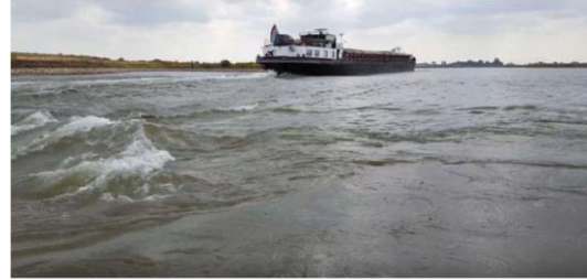
Figure 4. Video still of flow caused by ship sailing from the IJssel downstream of the bifurcation into the Nederrijn upstream of the bifurcation.
