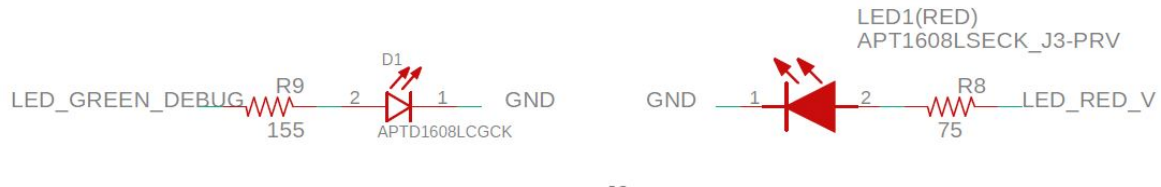
Figure 4.21: Schematic of prototype PCB MCU debugging LED's
