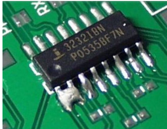
Figure 5.1: Example of solder bridge at IC [77]
