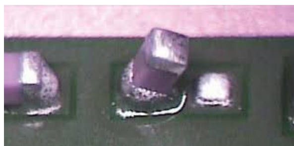
Figure 5.2: Example of tombstoning at a capacitor [78]
