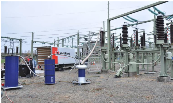
Figure 7.18: The DAC Diagnosis of Circuit B.
