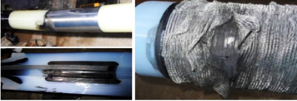
Figure 6.13: Faulty cable joint during inspection. Wrong positioning of joint housing caused a local PD activity and breakdown during DAC testing.
