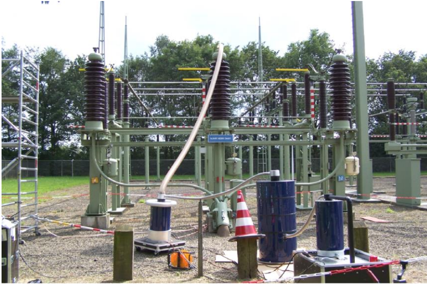
Figure 7.17: The DAC Diagnosis of the Circuit A.
