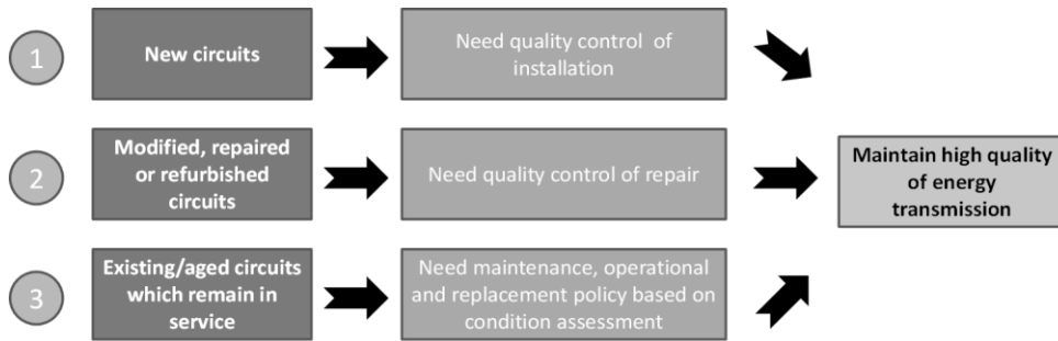
Figure 1.1: Approaches to maintaining power cable reliability.
