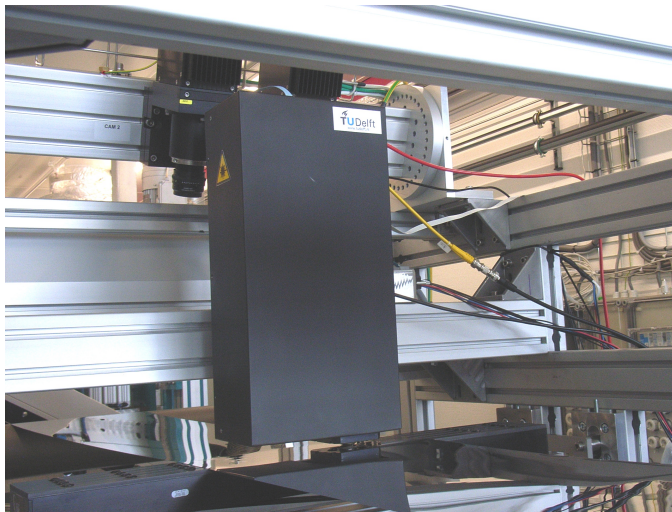
Figure 1.6: The prototype CFS particle detector installed in production line. The transparent of polymer substrate can be seen under it.
