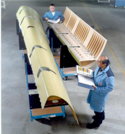
**Figure 2.11:** J-Nose of the Airbus A380 made from woven glass fibre/PPS composite material by GKN Aerospace [49]
