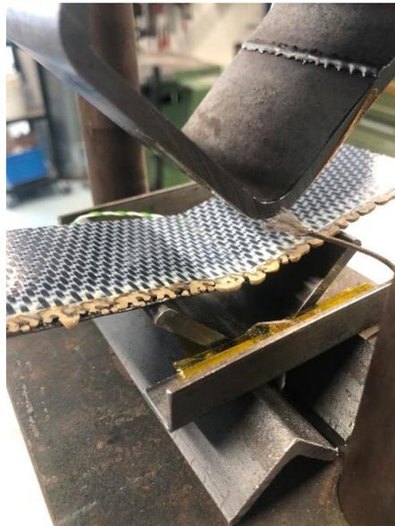
The partial bend sample did show an impression of the tooling, demonstrating that the material did have intimate contact with the tool. Throughout the forming process, cracking could be heard which indicated that the material was not at the processing temperature, and fibres were being broken due to elastic bending.
