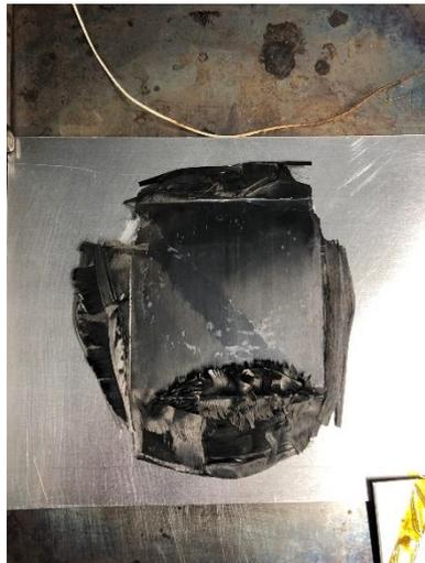
*Figure 3 Sample after pressing with the mould removed, showing signs that the material shifted during processing*
