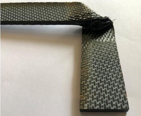
**Figure 6.44:** First fold made for the core part of the handrail
