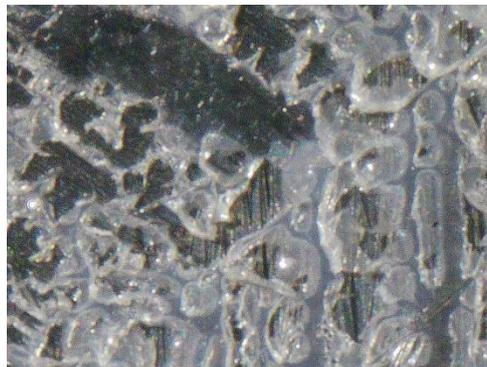
*Figure 5 Image taken from the microscope of the surface of the sample, demonstrating severe porosity*
