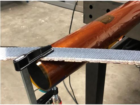
**Figure 6.41:** Setup of forming a curled section from a laminate off-cut, using a hot-air gun and a round steel stock
