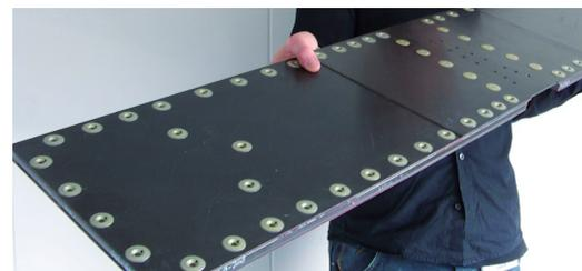
**Figure 2.20:** Pressure bulkhead floor panel for the G550 and G650 made from carbon fibre/PEI face sheets by GKN Aerospace [41]
