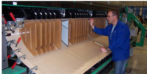
**Figure 3.4:** Local joining of the A380 J-Nose ribs with the skin using resistance welding [18]
