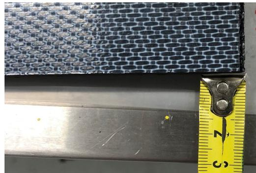
**Figure F.5:** Other end of the clamped laminate off-cut with the measurement of the in-plane warpage over its length
