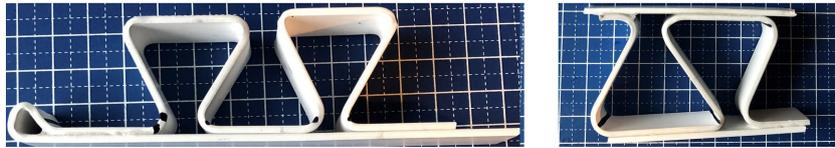
**Figure 5.12:** Two initial forms of the beam sandwich structure made from PVC strips
