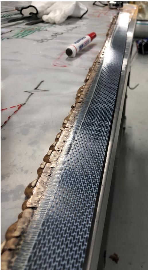
**Figure F.4:** Clamped end of the laminate off-cut to determine the in-plane warpage
