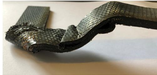
**Figure 6.45:** Single formed bends with a large radius made as a continuation of the fold
