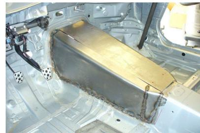
**Figure 5.6:** Possible application of a flat sheet, with local bends to comply to a certain form, as a structural element in a vehicle
