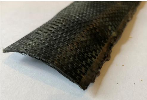
**Figure 6.46:** Top section of the handrail that is formed along the radius of the round stock
