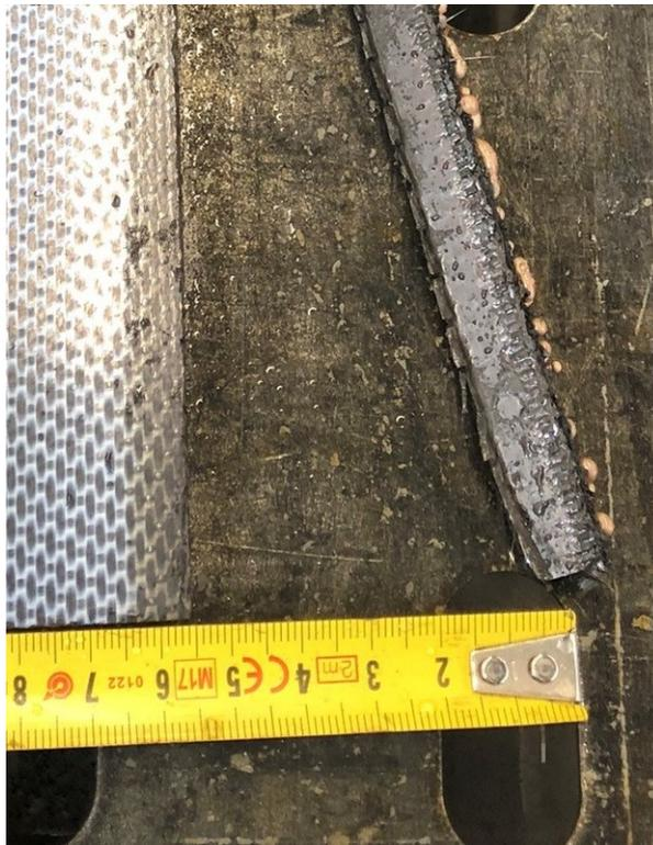
**Figure 6.34:** Laminate off-cut with the partially trimmed off residual matrix edge, demonstrating the curvature after trimming
