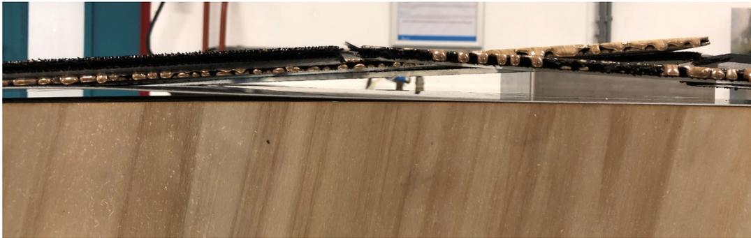
**Figure 6.33:** Close-up of the laminate off-cuts when placed on the curved wooden mould
