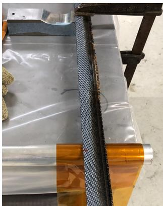
**Figure 6.39:** Setup of the single bend forming using a hot-air gun, to locally heat the material
