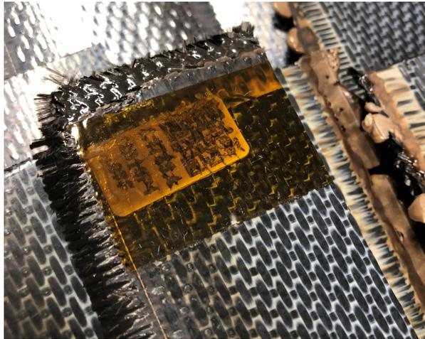
**Figure F.3:** Foreign material contaminants on the outside of the material, in this case PI tape (kapton) and a piece of paper
