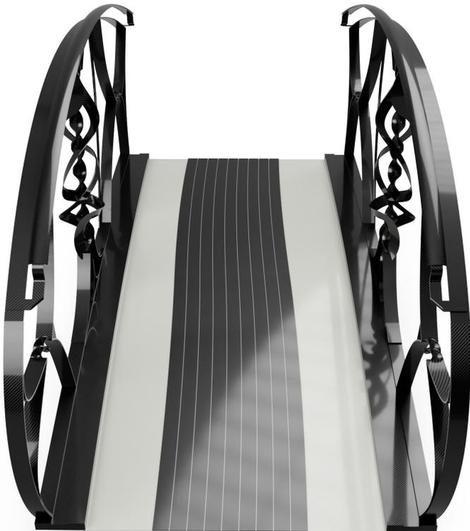
**Figure 6.52:** Top view of the bridge demonstrating the S shaped path created from the laminate off-cuts across the deck of the bridge
