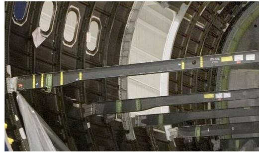
**Figure 5.8:** Composite floor beam of the Boeing 787 aircraft, demonstrating a step-wise beam height over the length of the beam [93]
