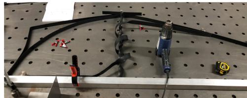
**Figure 6.38:** Thermoplastic strip material locally heated and bent into shape, keeping its form after the supports are removed
