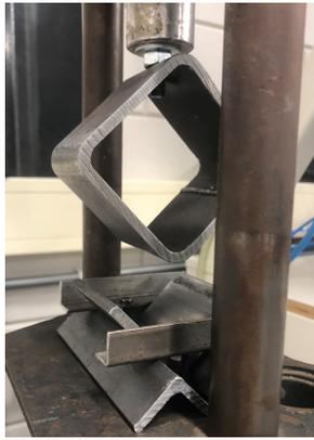
**Figure 5.14:** Tooling used for the experimental forming of single bends in the laminate off-cuts
