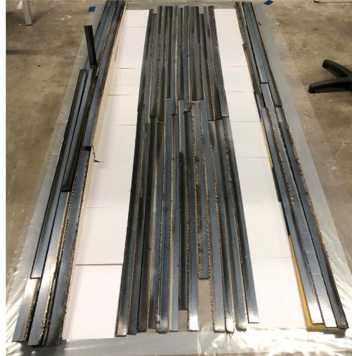
**Figure 6.36:** Slightly curved path made from the laminate off-cuts, with the white paper creating the contrast between the EOL WTB deck material
