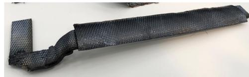
**Figure 6.47:** Assembled top curved and core part of the handrail, using double sided tape
