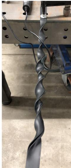
**Figure 6.43:** Thermoplastic strip shaped into a twisting pattern, using a hot air gun to locally soften the material to allow for twisting
