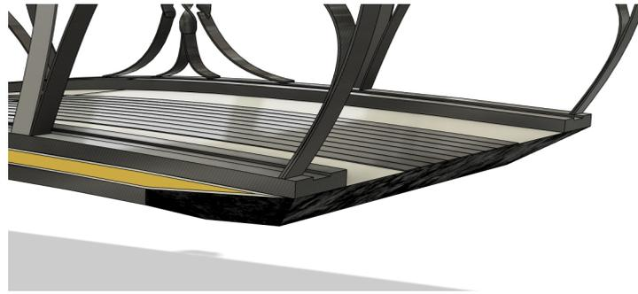
**Figure 6.48:** Abutment at the end of the bridge, designed to retract underneath the bridge to hide its aesthetics
