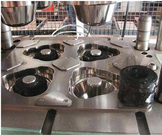
**Figure 3.8:** Example of a preform loaded into a forging mould [69]
