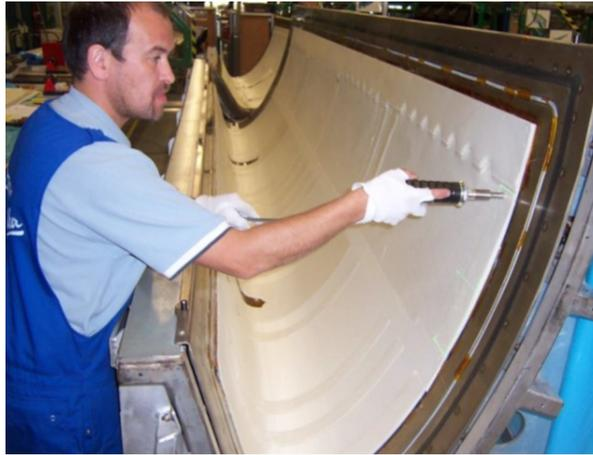
**Figure 2.22:** Layup process of the J-nose of the Airbus A380, using an ultrasonic spot welding tool [41]
