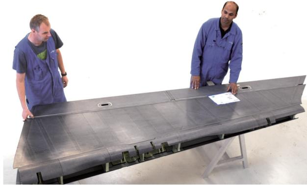
**Figure 2.12:** Vertical stabiliser of the G650 aircraft made from woven carbon/PPS composite by GKN Aerospace [41]
