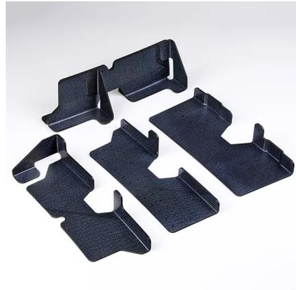
**Figure 2.35:** Complex formed parts after edge trimming [45][60]
