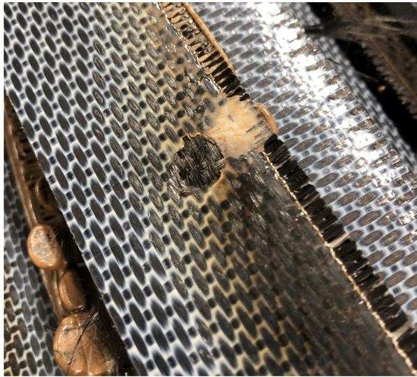
**Figure F.1:** Close-up of the dry spot caused by a possible alignment pin, with thermal degradation and resin-squeeze out present
