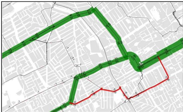
Fig. 3. Example of whatif results: the impact of a frequency increase of two PT lines on ridership (green = increase; red= decrease)
