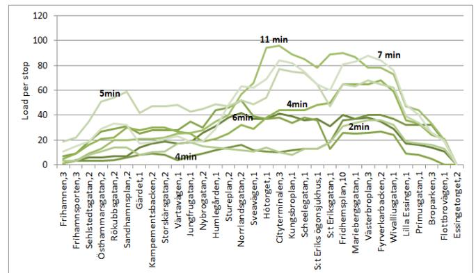
Fig. 4. Passenger loads on consecutive bus trips on the westbound direction of trunk line 1 in Stockholm and their respective headways
