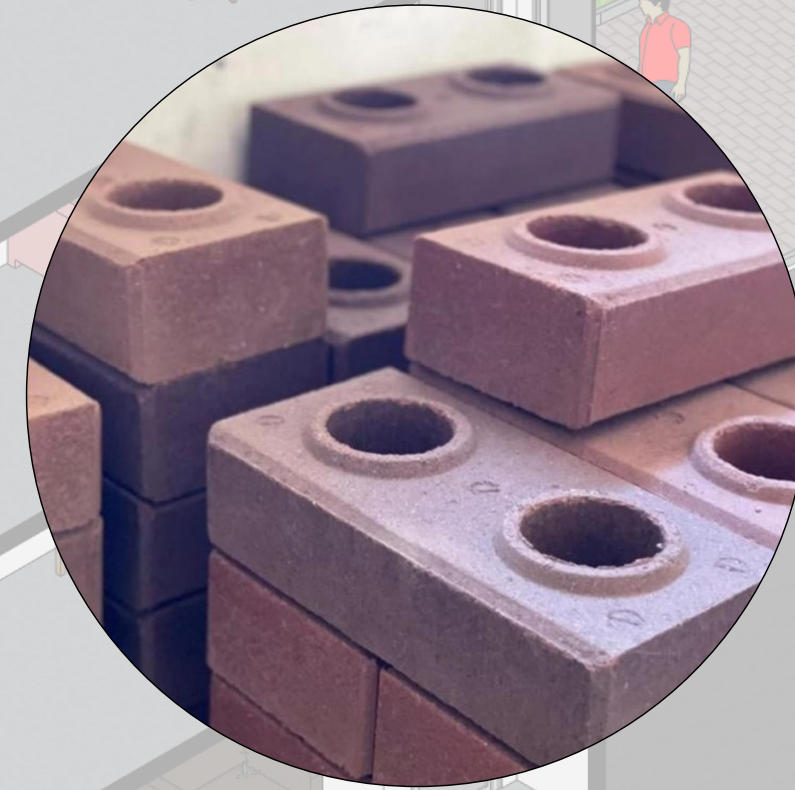
non-structural walls: ceramics + compressed earth blocks
