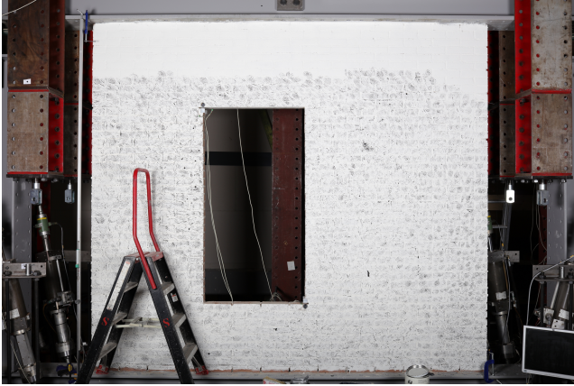
Figure 5. Photograph of one of the experimental walls, before the application of the DIC pattern has been finished.
