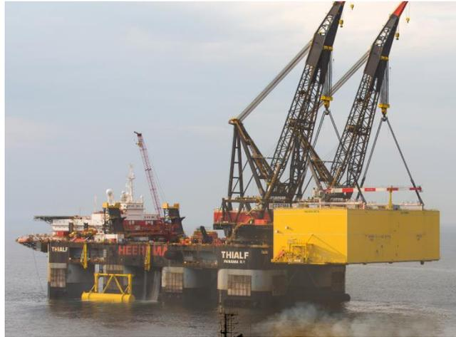
Figure 7.16: SSCV Thialf in dual lift mode(source: Siemens AG)
