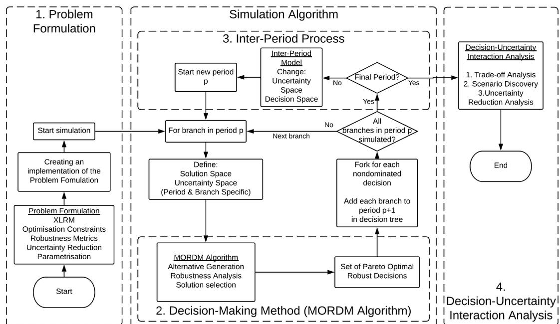
**Figure 3.4:** Flowchart of the Approach for Simulation and Analysis of the Interplay between Decisions and Uncertainty
