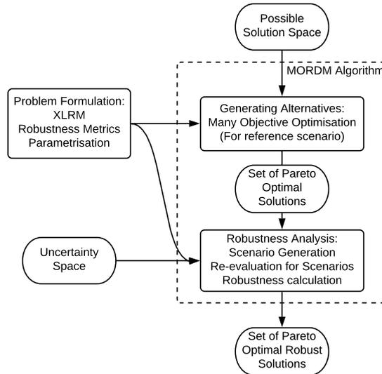
**Figure 3.3:** Many-Objective Robust Decision-Making Algorithm Design
