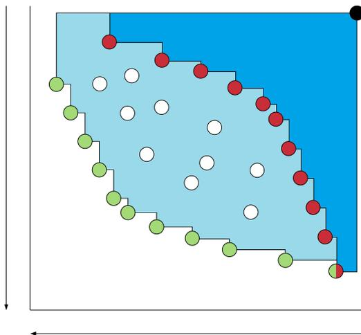
**Figure 9.1:** Illustration of a Pareto front and an inverse Pareto front
