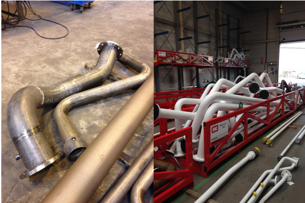
Figure 24 – Left : Pipe spool with bend and welded elbow
