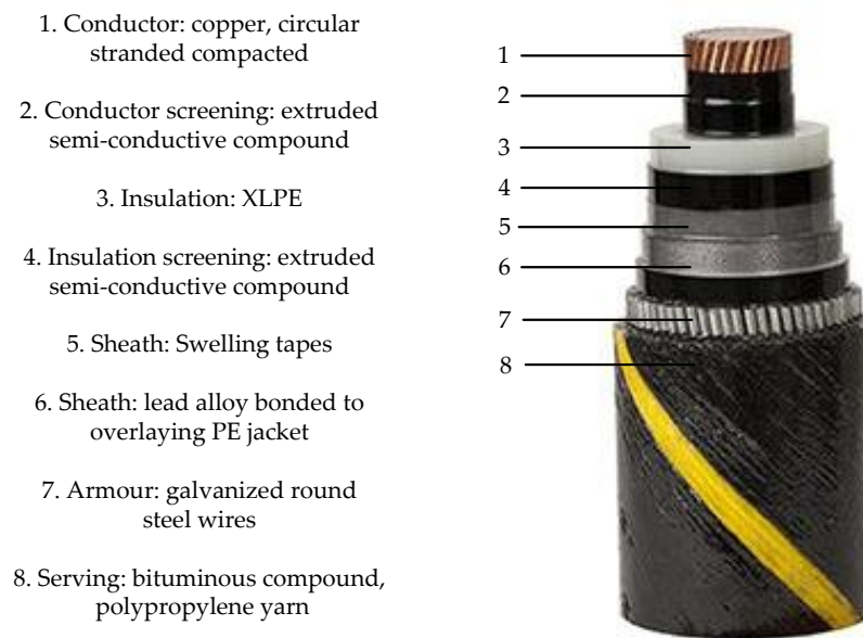
FIGURE 3.5: Typical design of a HVDC SPC with XLPE insulation (Courtesy of ABB) [14]
