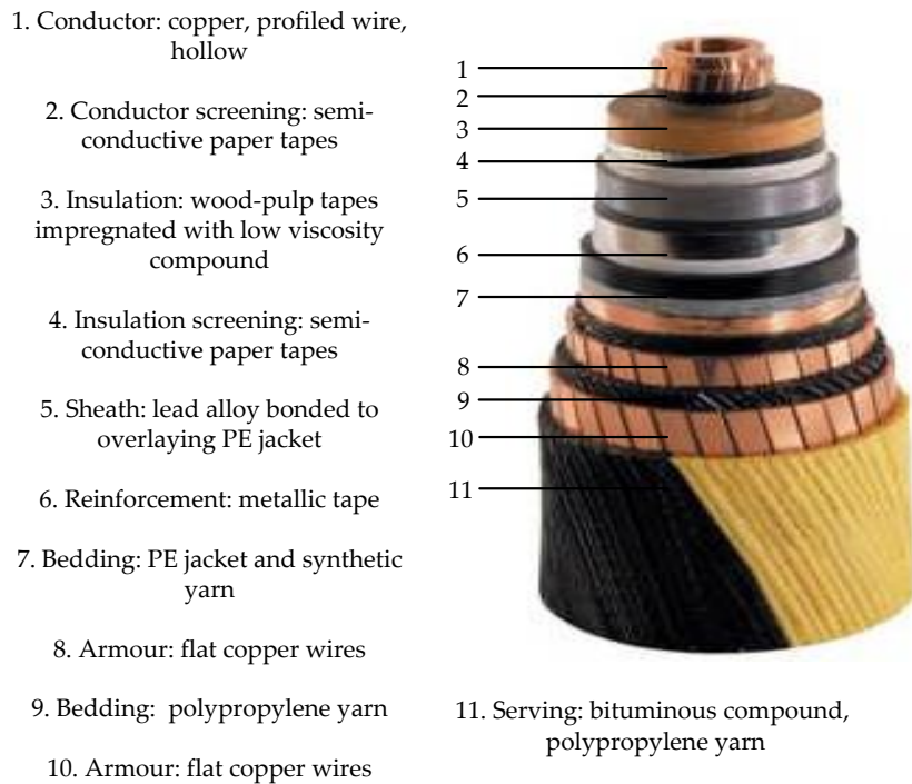
FIGURE 3.6: Typical design of a HVDC fluid-filled SPC (Courtesy of PRYSMIAN) [15]
