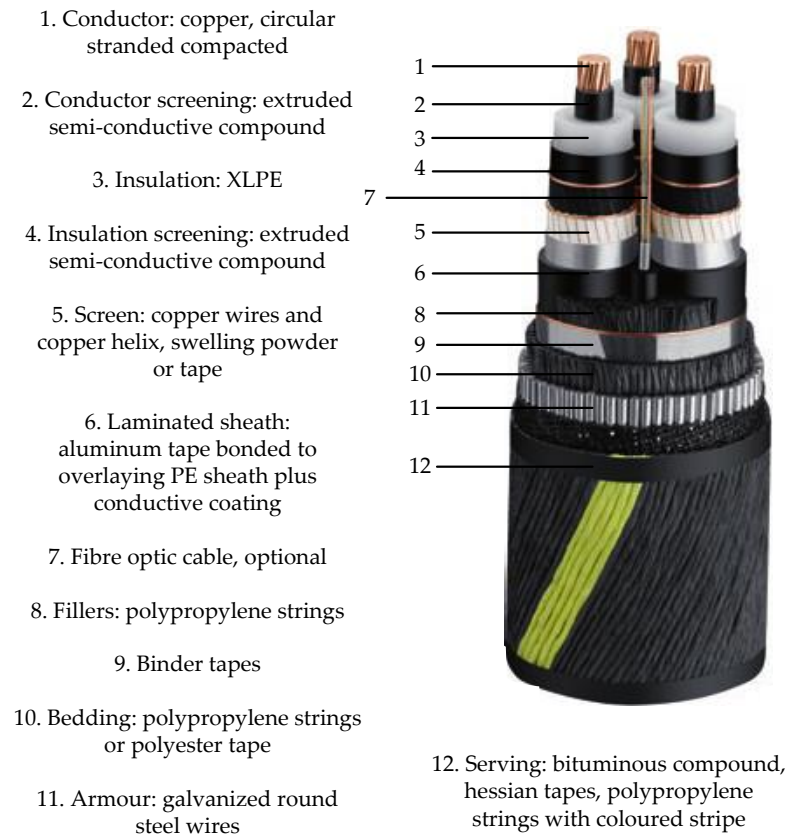
FIGURE 3.3: Typical design of a MVAC SPC with XLPE insulation (Courtesy of Nexans) [13]
