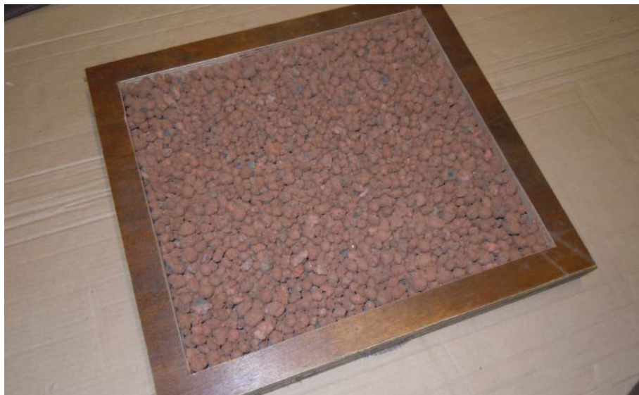
Fig. 160 Test element with hydro grains as absorption, (negative effect)
