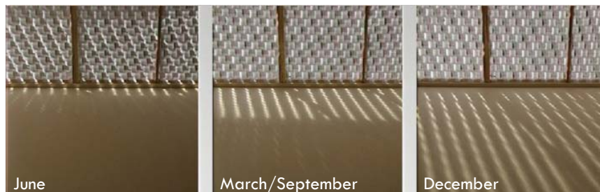
Fig. 145 Test model zig zag sunshading system
