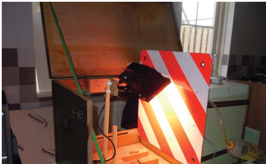
Fig. 156 Radiation (from light) provides negative cooling influences
