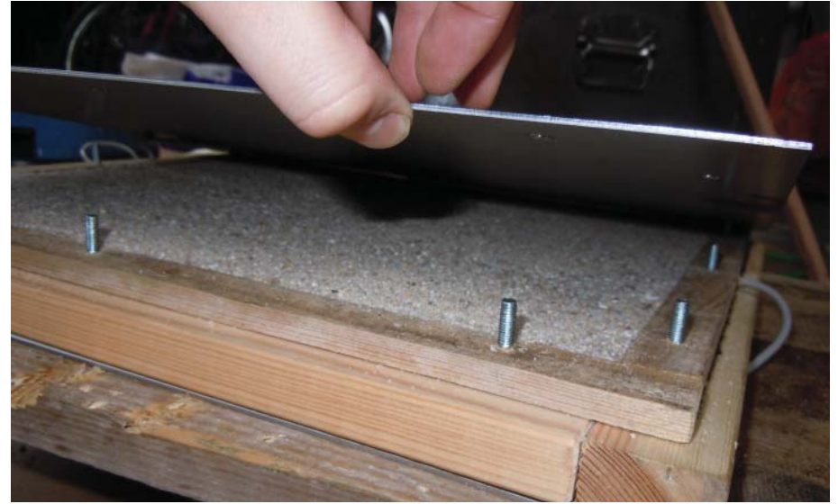
Fig. 159 Absorbion layer behind metal plate
