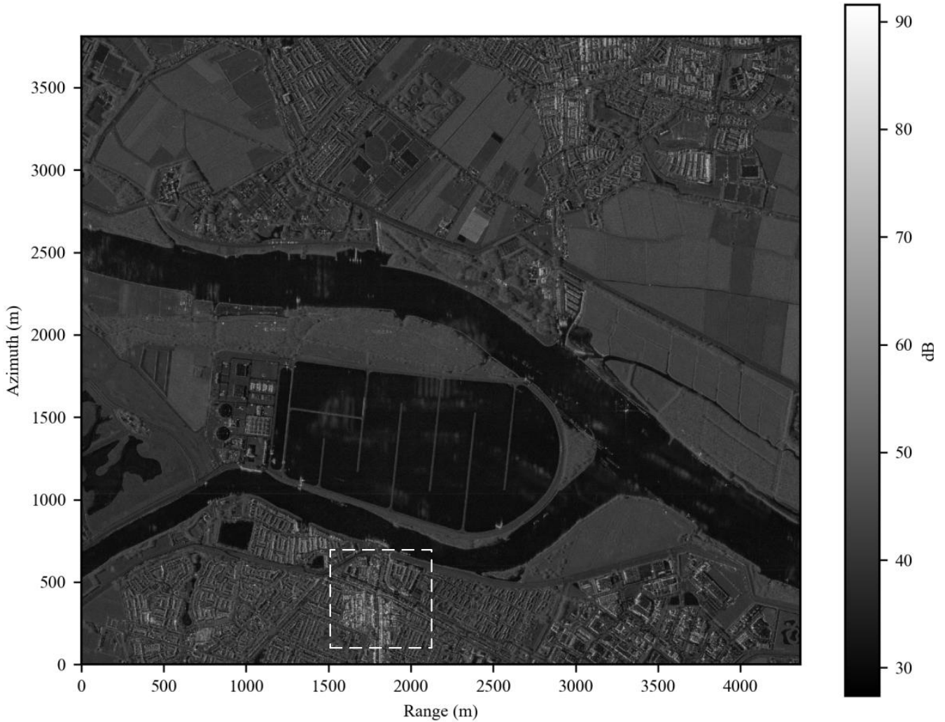
FIGURE 5. Squared mean intensity image of the original TerraSAR-X stack. We can observe several kinds of terrain, including urban areas, water, and grassland, from the varied scattering characteristics. The part marked by the dashed line is shown in detail in Figure 11.
